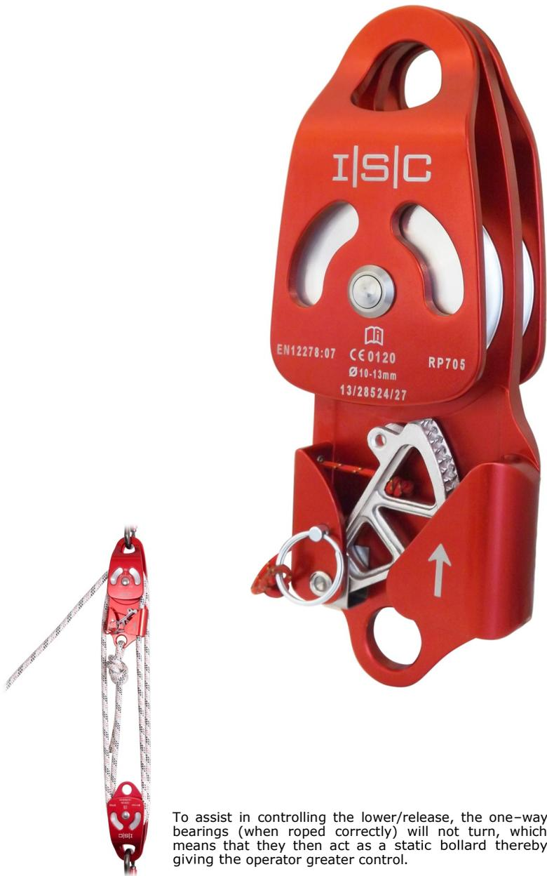
To assist in controlling the lower/release, the one-way bearings (when roped correctly) will not turn, which means that they then act as a static bollard thereby giving the operator greater control.
